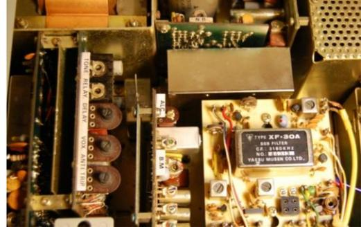
Audio board on the left, undo the screws and it pulls out
